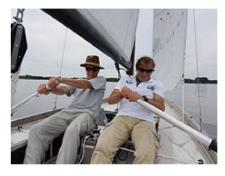
The aluminum-hulled LelieClass has a 2.20m beam, weighs 550 kilos (1,212lbs.) and is uncomplicated. The mast can be lowered quickly, an outboard engine can be attached to the double-walled transom. There is room for 5 adults. It can be equipped with a stem-to-stern tent on 3 aluminum poles which makes it possible to sleep under and on the foredeck.
